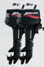
Engine Type:2-Cyl 169ccWeight:26kgSteering:Tiller (Side shift)Starting:ManualGear Shift:F-N-RTrim Positions:6Shaft Length:15"(M), 20"(L)
